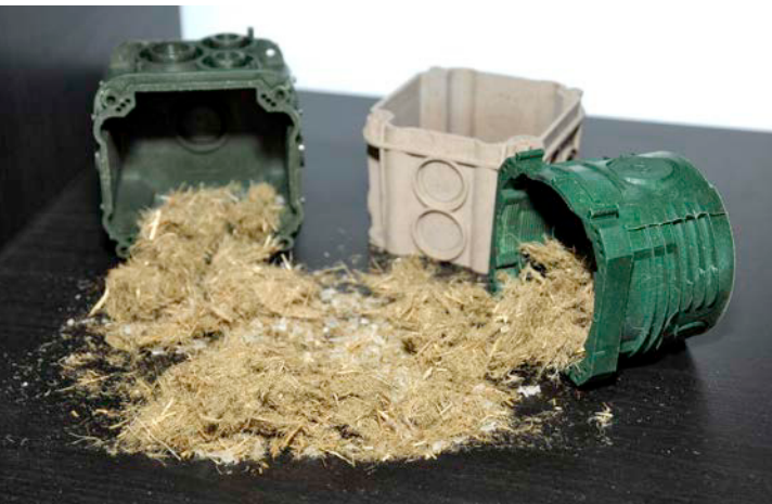
Flush-mounted boxes made of bioplastic. The fibers made from meadow grass exemplify the ecological component of the product.
